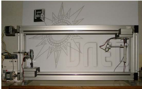
Figure 7. Didactical setup of the thin lens experiment
